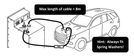
**B&S 4** Cable is recommended to connect the Vehicle Battery to the ToughPower.
