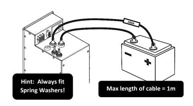
**B&S 2 Cable**, at no greater length than **1m**, MUST be used to connect the Dual (Auxiliary) Battery to the ToughPower. Performance at High Current outputs will be compromised if these cables are longer or are a thinner gauge.
