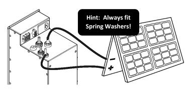
Fit M6 & M8 Ring Terminal Connectors to your Solar Panel cables to attach to the ToughPower Terminal Posts.
