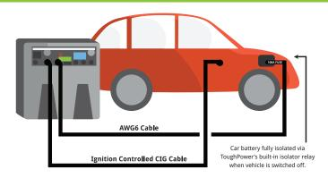
Simply connect the ToughPower to your car via an ignition controlled CIG socket and an AWG6 cable connected to your vehicle's battery (with 100A fuse), turn the ToughPower on, and let the ToughPower handle the rest!
